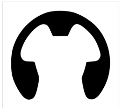
Lock washer according to DIN 6799, which is also referred to as an "E-ring" due to a certain similarity to the letter "E" or "e".
