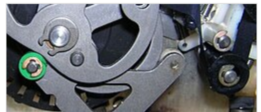
Machine part with four external locking rings. The brass-colored, clip-on locking washers are often referred to in the trade as E-rings. The large circlip ("Seeger ring") can be opened with circlip pliers.
