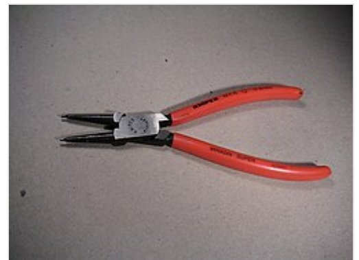
Circlip pliers with pointed ends for installing internal circlips
