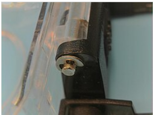
E-ring on the axle of an action cam housing
